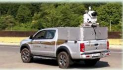
3D - mobile mapping technology, which is one of the modern trends in the field of application of Information Technologies in Distribution Networks, has already been put into use for more accurate and flexible implementation of operation, registration, analysis and planning of Electric networks.
